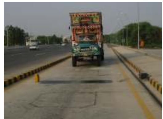
Truck approaching through WIM lane and passing over SSWIM in-road sensors
