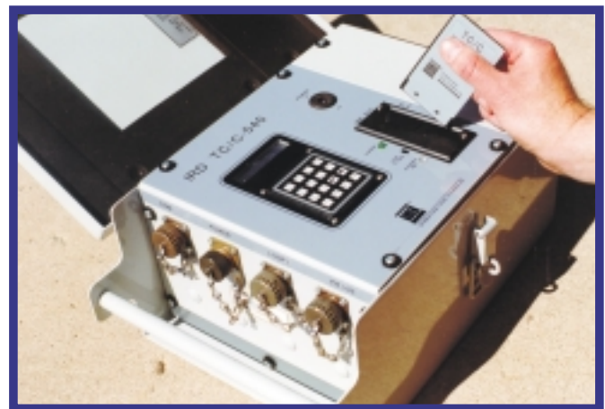
TCC Traffic Data Collection Unit
